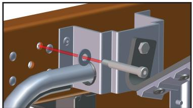
5. Insert the (new) Socket Head Bolt through the (new) 5/16" Washer and into the rail, as shown in the illustration.
