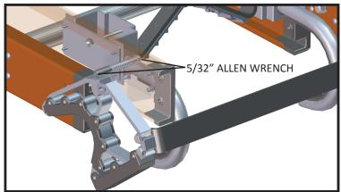
3. Using (2) 5/32" Allen Wrenches, loosen the Push Pin and the Socket Head Bolt.
