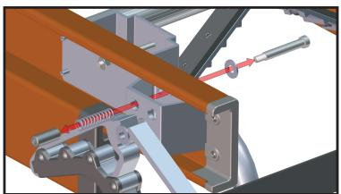
4. Remove and discard the Socket Head Bolt, Push Pin, Locking Spring and 5/16" Washer.
