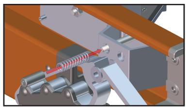
6. Insert the (new) spring and Push Pin onto the (new) Socket Head Bolt, as shown in the illustration. Tighten using (2) 5/32" Allen wrenches.
